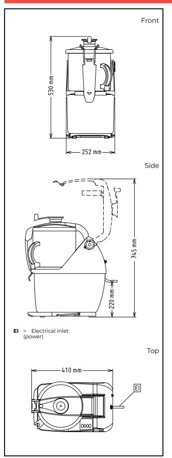
Electric Supply voltage: 200-240 V/1N ph/50/60 Hz Capacity: Performance (up to): 550 kg/Cycle 7 litres Capacity: Key Information: External dimensions, Width: 252 mm External dimensions, 485 mm Depth: External dimensions, Height: 505 mm **Shipping weight:** ISO 9001; ISO 14001 kg
